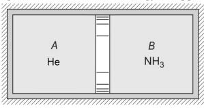
such that ammonia expands and slowly compresses the helium to a pressure of 600 kPa. The compression of helium follows a process with an index of 1.667. Find a) the volume (m<sup>3</sup>) of helium in the final state, b) work done by ammonia (kJ), and c) the final temperature of ammonia (°C).
