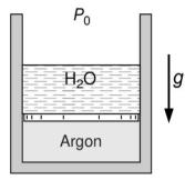
below the thin insulated piston of mass 20 kg as shown in the figure. Heat is supplied to the argon such that the piston rises and pushes the water out over the top edge. Find a) the work done to remove the whole water from the top of the piston (kJ), b) the heat transfer to the argon during the process (kJ), and c) plot the process in a *P*-*v* diagram for the argon. Assume atmospheric pressure as 101 kPa and ignore piston thickness. [20M]
