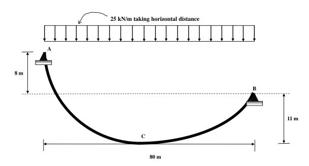
Q.3. Find the vertical force and bending moment at point B for the following 3-hinged arch. Equation of the shape of the arch is  $y = 0.06666(x - 15)^2$ . [10]
