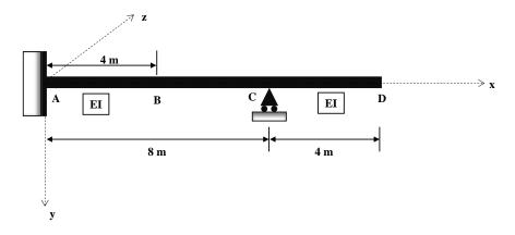
Q.6. Analyze the following beam using moment distribution method. Find all the reactions and BM at B.
