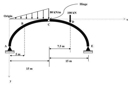
Q.4. Solve the frame by force method. Find the reactions. Draw the shear force and bending moment diagrams mentioning the values. [15]
