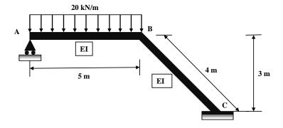
Q.5. Draw the influence line diagram (I.L.D) for bending moment at B of the following beam. Use Müller-Breslau principle. Find the ordinates of the diagram at every 2m. El is constant throughout the beam.
