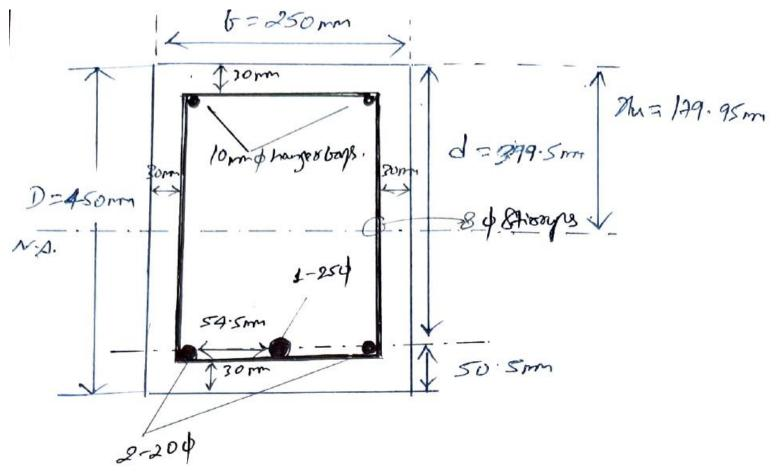
Assuming that the c.g. of reinforcement group passes through the center of 25 mm bar,
