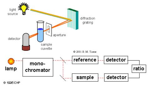
Single beam UV Vis spectrometer  $\,$  - instrument is calibrated with a reference cell containing only solvent to determine the I<sub>o</sub> value necessary for an absorbance measurement
