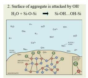
3. Silanol groups (Si-OH) on surface are broken down by OH<sup>-</sup> into SiO<sup>-</sup> molecules
