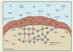
6. When the expansive pressure exceeds the tensile strength of the concrete, the concrete cracks
