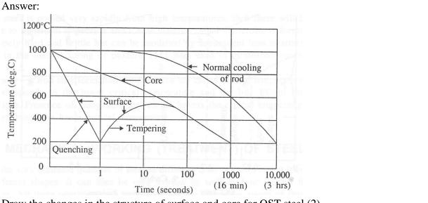
c) Draw the changes in the structure of surface and core for QST steel (2)
