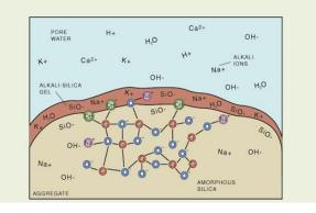
5. Alkali-silica gel takes in water, expanding and exerting a force against surrounding concrete.
