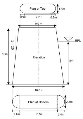
**Q6.** The geometrical details of a square concrete tank are:
