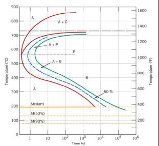
h) Quench to 650 °C (1200 ° F), hold at this temperature for 3 s, quench to 400 °C (750 ° F), hold for 25 s, then quench to room temperature.
