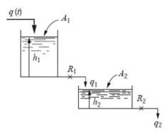
3. Develop the closed-loop transfer function for the system shown in Fig.
