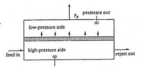
b. It is proposed to use membrane for separation of  $CO_2$  from biogas ( $CO_2 = 40 \text{ mol}\%$  and  $CH_4 = 60 \text{ mol}\%$ ). A membrane has a selectivity of 5 for  $CO_2/CH_4$ , determine the maximum  $CO_2$  concentration that can be obtained for a single stage device shown in the (a).
