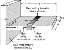
The ambient temperature is 30°C and the temperature of the wall is 100°C. The heat transfer coefficient (h) is 5 W/(m<sup>2</sup>.°C). The thermal conductivity (k) of metal is 400 W/(m.°C). The thickness (2B) is 4 mm.
