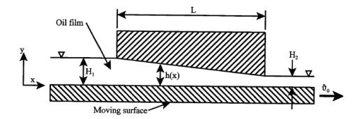
As shown in the above figure, a simple slider bearing has a uniform taper from the inlet, where the gap is  $H_1$ , to the exit where the gap is  $H_2$ . This gap is filled with oil of viscosity  $\mu$  and density  $\rho$ . The upper surface is stationary and the lower surface moves at a steady velocity  $v_0$ . The thickness of the oil film at a location x measured relative to the leading edge of bearing is h(x)
