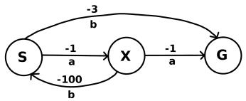
State S is the starting state and state G is the terminal state. Each state has two possible actions : a and b. Action values for the terminal state (i.e.  $Q(G, \cdot)$ ) are initialized to 0. The remaining action values are initialized to arbitrary values. The discount rate  $(\gamma)$  is .8.
