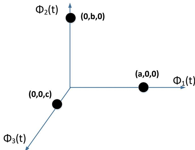
Q4. A two-dimensional constellation is shown in the figure. All symbols are equi-probable and the distance between each adjacent symbol is 2.
