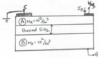
(i) Predict the polarity of V<sub>G</sub> to create depletion charge in the B region and also find the suitable thickness of region A to ensure 10 nm channel from S to D in case region B develops a 10 nm depletion region.
