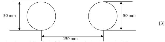
Q.2 Find the view factor of the spherical ring as shown in the figure to itself  $F_{1-1}$ .
