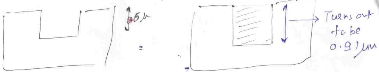
Groove is of 0.5 μm.
