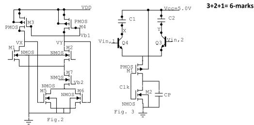
3. the equivalent circuit of Fig 3, assuming the input CM-level ≈ V<sub>CC</sub>, V<sub>BE</sub> and R<sub>on-M1</sub> to be constant. Estimate the small signal voltage gain at t = ∞, if V<sub>BE</sub> = 0.7V, 2C<sub>p</sub>=C<sub>1</sub>=C<sub>2</sub>=10 pf.
