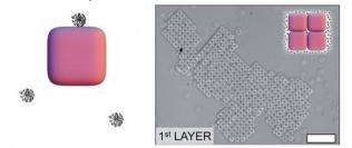
The cubical SiO2 particles of size 1  $\mu$ m form a crystal when polyethylene oxide (PEO) molecules of size 50 nm are added. Explain why this happens and describe the physics of the process. (3)
